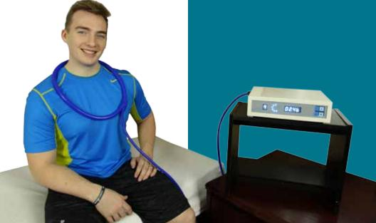
The Curatron FLASH stores enormous amounts of energy at a very high voltage in a supercharged capacitor which is discharged by a very high voltage and very high current solid state semiconductor with under precise computer control into the PEMF coil.
